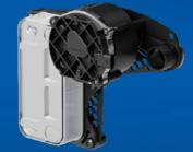
**Oil management modules** integrate multiple components and system functions in a very compact environment. Beside the electrical oil pumps further components can be integrated such as heat exchangers, filters, check valves, sensors, and oil pan. Due to the deletion of many unnecessary pipes, interfaces, brackets and the usage of plastic compound materials oil management modules can enable significant weight reduction.
