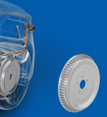
Lightweight hybrid brake drum consisting of grey-cast-iron friction ring and aluminum housing saves up to 40% weight compared to standard brake drums.
