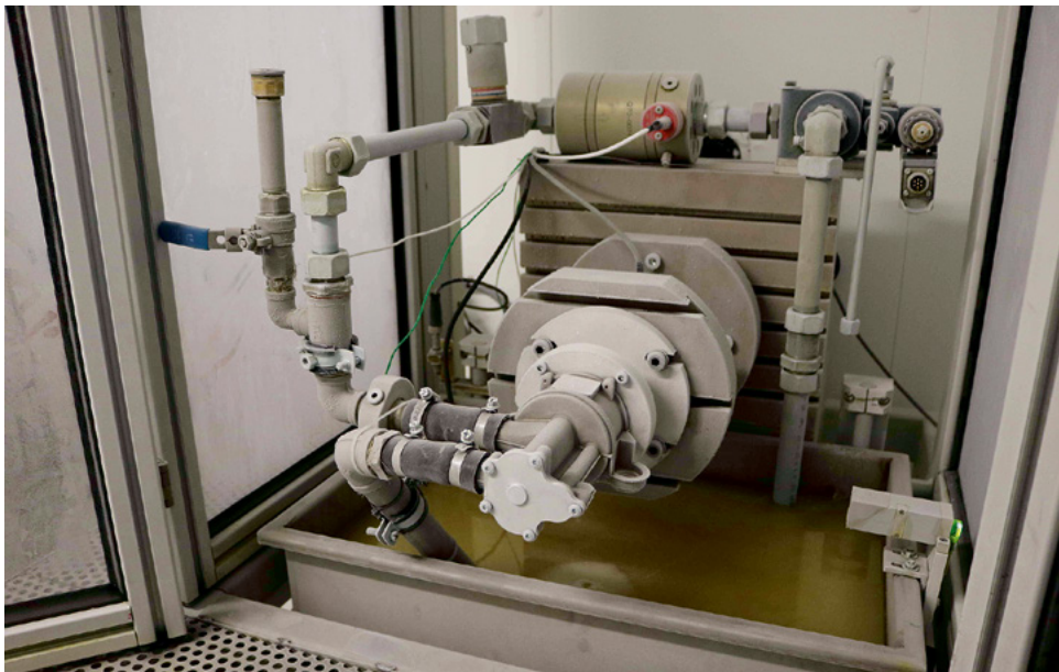
FIGURE 4 Test setup for measuring the starting torques of the pumps in the refrigeration chamber at -30 °C (© SHW)
