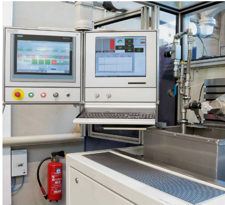
FIGURE 1 Test setup for measuring the pumps on the oil pump test bench (© SHW)
